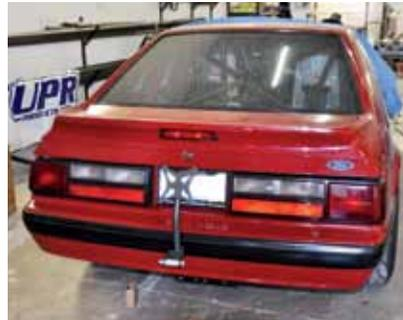
▲ Dave at Tig-Vision is a bit of a perfectionist. After installing the mini-tubs and relocating the coilovers, he painted the wheelwells black, painted the axle housing silver, he even powdercoated the parachute mount. Tig-Vision custom fabricated this parachute mount to bolt right onto the factory bumper mounts, and the upright portion is completely removable if we choose to roll incognito.
