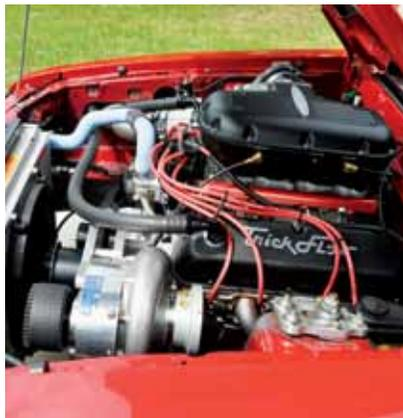
▲ Although Project Shocker is in fact a street car and we still have an inlet air filter for our ProCharger F-1R, we are determined to squeeze every last bit of horsepower out of this 428 stroker, so we ordered an inlet bell from ProCharger. It is said to increase max boost by as much as 2 psi with no other changes, and we'll take any advantage we can get! Any guesses on how much power Project Shocker will make on the dyno?
