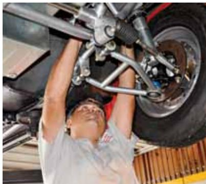
▲ Our next stop was Segura Automotive in Fort Myers, Florida, where Owner, Lead Tech, and accomplished True Street racer Chris Segura assembled our braking system. In the process of upgrading to Strange Engineering Pro Race brakes, we replaced every component of the braking system. Here, Chris has already fabricated the rear brake lines and he is connecting the front lines.
