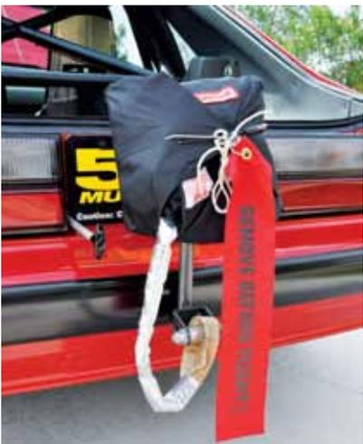
▲ We installed this Simpson Skyjacker parachute from Summit Racing Equipment and the battery cutoff switch in order to satisfy NHRA safety inspectors. However, both the parachute mount and the cutoff switch handle are easily removable for low-key street driving.
