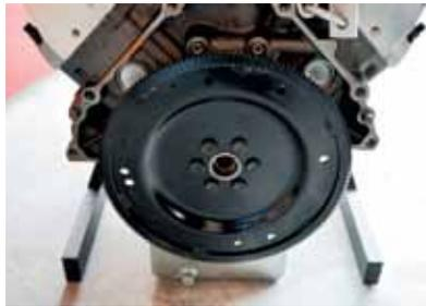
▲ Next we used ARP hardware to bolt the SFI-certified 157-tooth JW flywheel to our 428-inch stroker.
