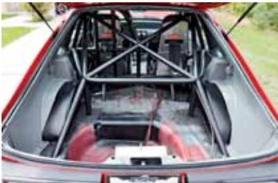
▲ Project Shocker looks fairly serious with the hatchback opened to reveal its Rogue Race Cars roll-cage and Tig-Vision mini-tubs, but new carpet and a custom rear-seat delete will return the Shocker to its show-car standards.
