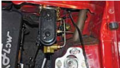
▲ This Racecraft Inc. manual brake conversion kit includes a Strange Engineering master cylinder and offers the correct pedal pressure for our manual brake setup. The front brake line is directly connected to a TCI RollStop Kit. TCI's RollStop Kit, which is activated by a button on the TCI Outlaw Shifter, will allow the driver to hold the car in place while doing a burnout to heat up the tires. It is a breeze to operate, and the solenoid valve only uses 1 amp of current.
