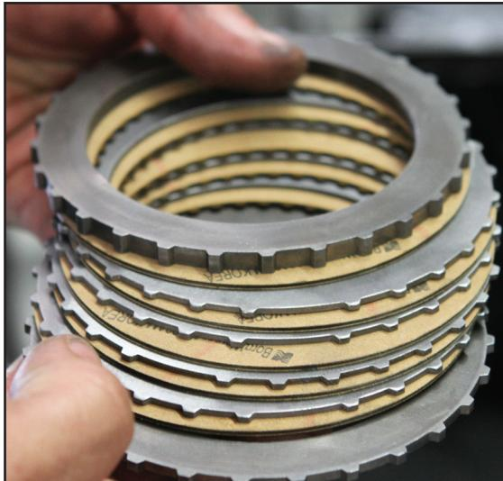
>> The forward drum uses Borg Warner clutches and OEM steel plates. The reason is, that once these clutches are applied, they stay applied. Apuzzo told us that it isn't like these are shifting clutches that get beat up since they remain applied all the time.
