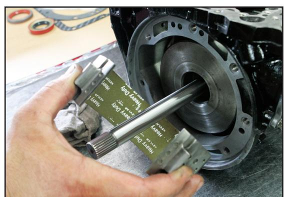
>> A Kevlar band for the forward drum is standard and a Redline version is optional.
